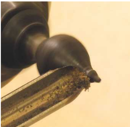
▲ Pic.31 After cutting off the finial, grip its spigot in a chuck to finish the pointed end. Les is using a Jacobs'-style chuck in the headstock; this works perfectly on small work like this
